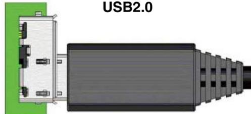
In case of USB 2.0 transmission + charging, conventional Micro USB 2.0 plug is usable.
