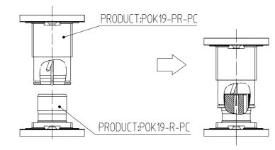
Non-combine or product damage due to primary deformation
