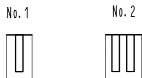
Figure-1 contact No. marking (10:1)
