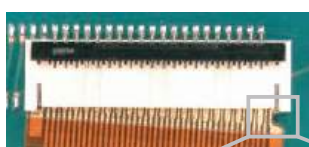
Incomplete FPC Insertion
