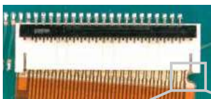
Incomplete FPC insertion
