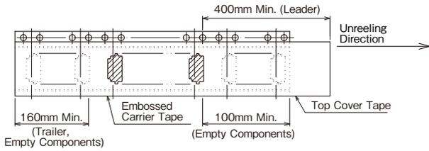
Note 1 : The package complies with JIS C 0806 and IEC 60286-3 (Packaging of components for automatic handling).
