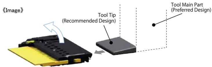
Pull out the FPC horizontally after releasing the actuator lock.
