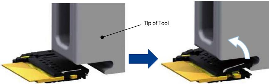
(2) The customer can design the actuator lock removal tool as preferred.
