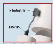
Robot to Camera Connection Example
