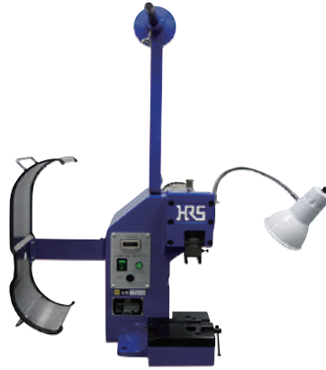
Automatic Crimp Tool CM-105C
