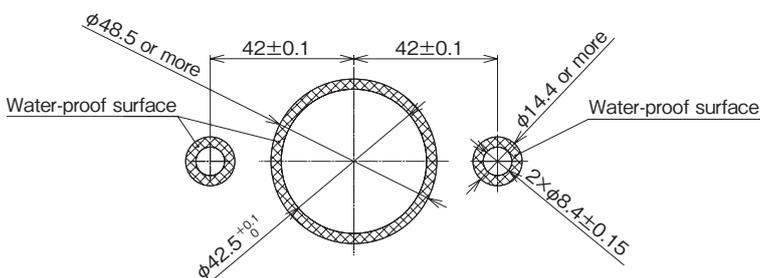
Recommended panel thickness  $t=2$  to 4.5mm
