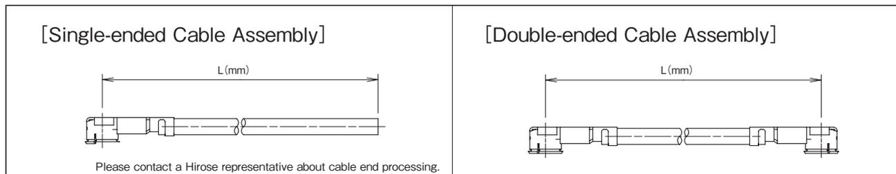
Note : Designate the dimensions from the center of the connector for both single-ended and double-ended cable assemblies. (Please write length L in mm.)
