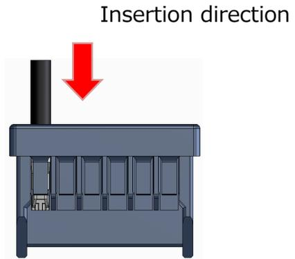
•To maintain performance reliability, do not tilt crimped contact (DF51K-\*\*\*\*SCF(A)) for insertion.
