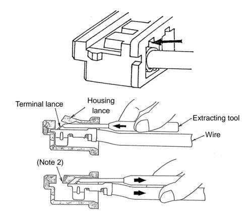
(Note 2) If you notice that the tip of the housing lance has scraped away when you pulled the terminal out, do not reuse the connector.
