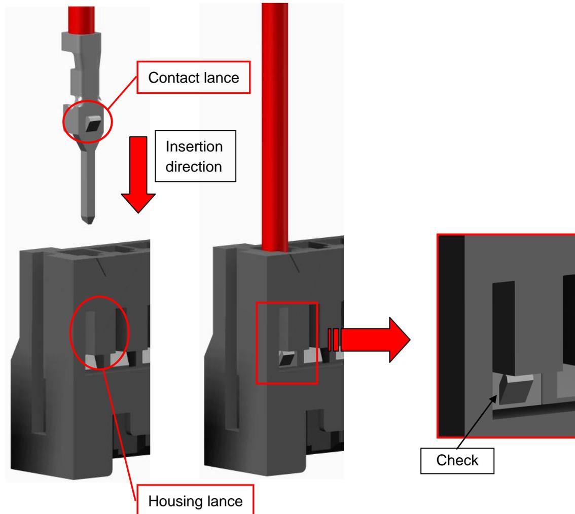
**NOTE: Repairing the crimp contact**
