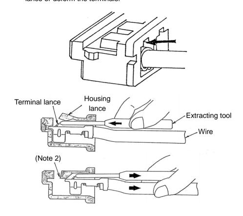
(Note 2) If you notice that the tip of the housing lance has scraped away when you pulled the terminal out, do not reuse the connector.
