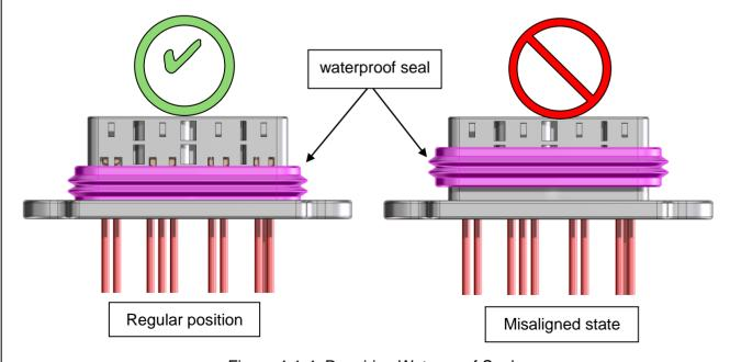
Figure 4-1-4. Repairing Waterproof Seal
