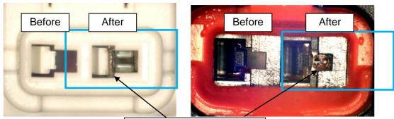
After Insert, Mold Lance Hidden by Crimp Terminal
