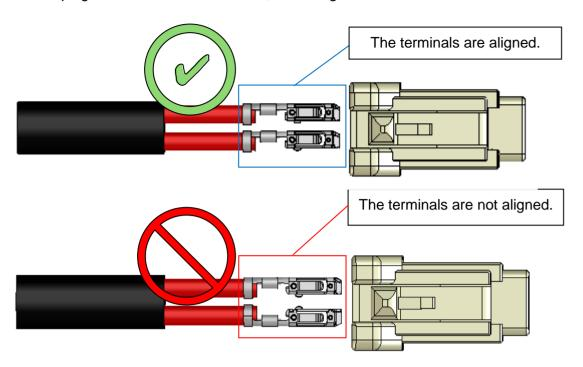
Figure 5-2. Terminal binding direction
