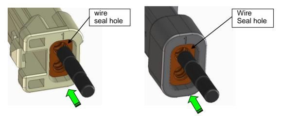
Figure 3-6-1. Inserting waterproof pin
