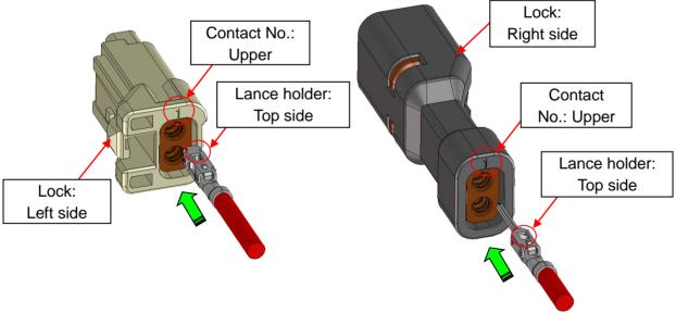
Figure 3-3-1. Before inserting the terminal
