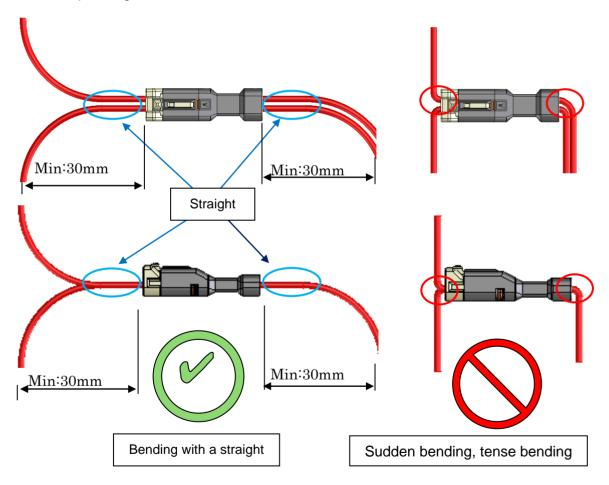
Figure 5-3. Cable bending
