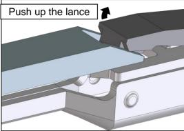
Figure 3-5-4. Crimp terminal pull-out
