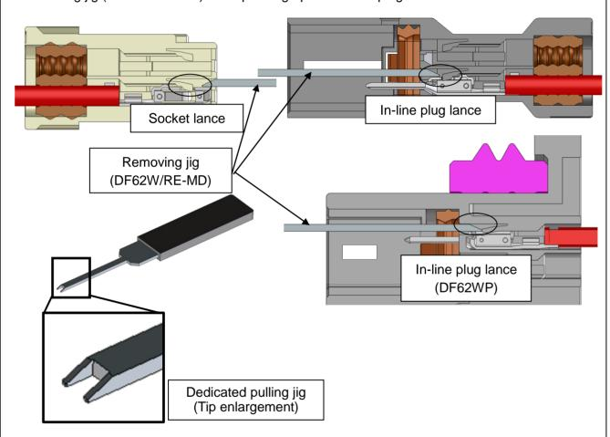
Figure 3-5-1. Schematic diagram
