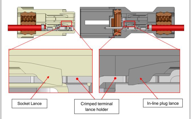
Figure 3-3-5. Checking the lance
