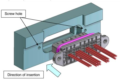
Figure 4-1-1. Insertion into panel
