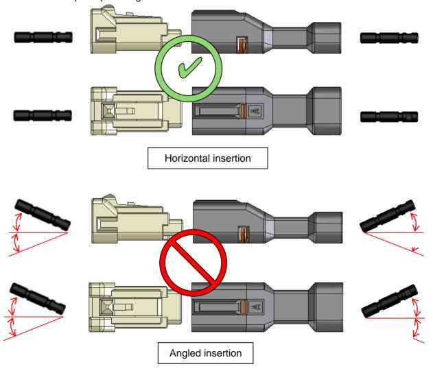
Figure 3-6-3. Prohibition of diagonal insertion of waterproof
