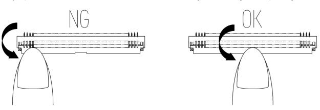
♦ Confirming the state of the lock Once it is locked, make sure that the actuator is parallel to the board. However, if the actuator approaches 0 degrees, make sure that it is not.
