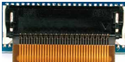
FPC is not inserted deep enough.
