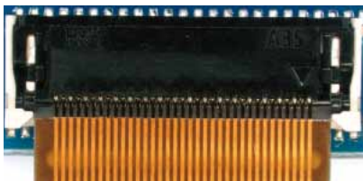
The outer shapes of FPC and the lock lever are parallel and inserted to the end.
