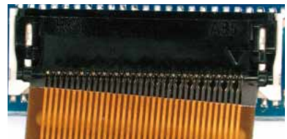
FPC is inserted diagonally.
