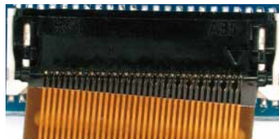
FPC is inserted diagonally.
