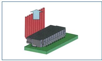
Robust design prevents damage while wire routing.
