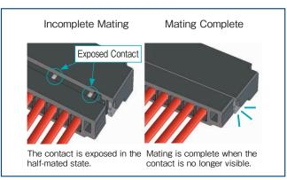
Allows for visual inspection of the mating process (The mated condition can be visually checked)
