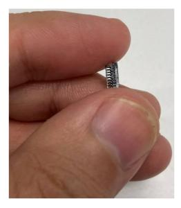
2) Hold the tip side of the crimp contact and insert it into each terminal hole of crimp case.
