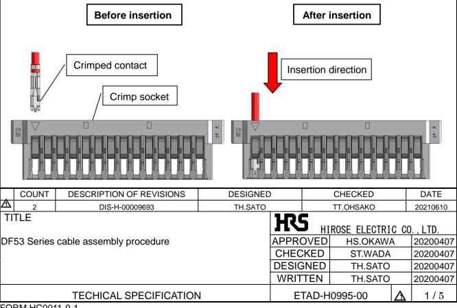
**A**[References] Procedure for inserting into the crimp case.
