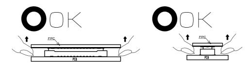
UN-MATED PARALLEL IT CAN BE REMOVED DIAGONALLY FROM THE PITCH DIRECTION.
