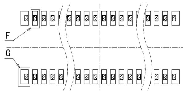
▨ Connector lead on PAD layout
