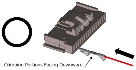
Note 1: Holding the cable, please insert straight into the housing.
