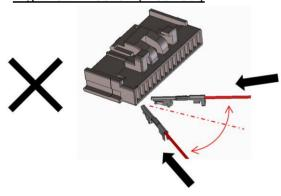
Scoop and twisted insertion (Incorrect)
