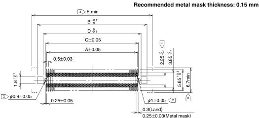
Note The cross-hatched area inside the SMT land may come into contact with the connector contacts and thus care should be taken that the pattern does not extend beyond the SMT land width.
