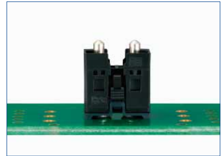
③ Interposer Installed
