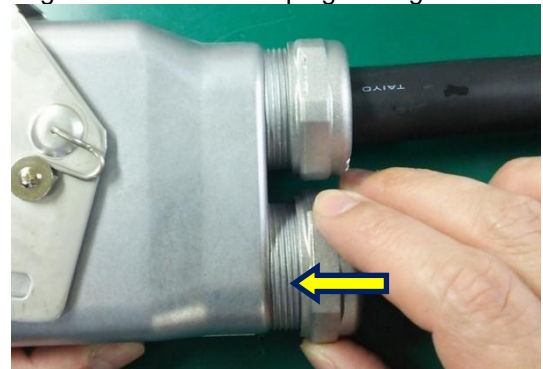
Signal side End bell cap tightening
