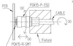
\* This product should be fixed with fixture so that it does not rotate vertically and horizontally when it is combined with mating material.
