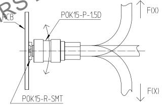
\* If you use this product without the fixing structure, If the force acts in the direction differently from the center of the product, it may cause the loss of function due to eccentricity of the product.
