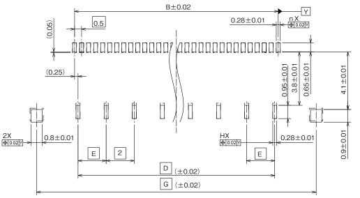
Recommended PCB Mounting Thickness : 0.12 Note : 'n' indicates the number of positions.
