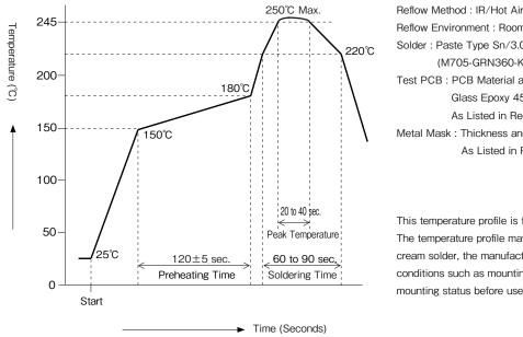
Reflow Environment : Room Air Solder : Paste Type Sn/3.0Ag/0.5Cu (M705-GRN360-K2-V made by Senju Metal Industry Co.) Test PCB : PCB Material and Size Glass Epoxy 45×25×1mm As Listed in Recommended PCB Mounting Pattern Metal Mask : Thickness and Opening Size As Listed in Recommended Metal Mask Dimensions
