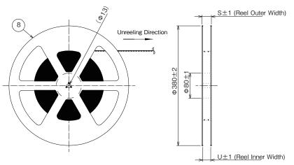
Note : The package complies with JIS C 0806 and IEC 60286-3 (Packaging of components for automatic handling).
