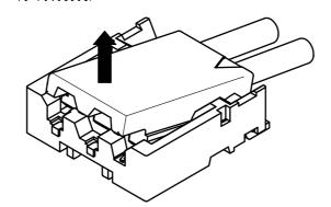
Blift up to the upper direction and positive lock is released. Removal completes.
