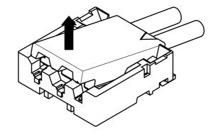
③Lift up to the upper direction and positive lock is released. Removal completes.
