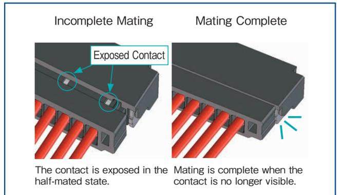
Allows for visual inspection of the mating process
