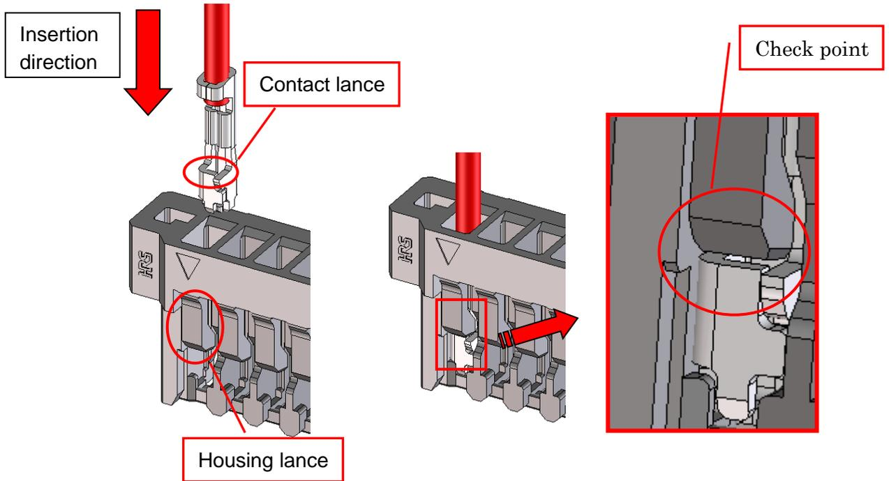
NOTE: Repairing the crimp contact
