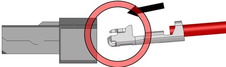
Angled insertion (Upward) (Incorrect)
