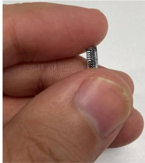
2) Hold the tip side of the crimp contact and insert it into each terminal hole of crimp case.
