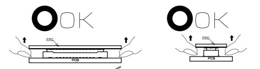
(2) IF THE CONNECTOR CANNOT BE UN-MATED PARALLEL IT CAN BE REMOVED DIAGONALLY FROM THE PITCH DIRECTION.
