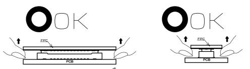
(2) If the connector council be un-mated parallel it can be removed diagonally from the pitch direction. Be careful to do so since this action applies stress on the contact.
