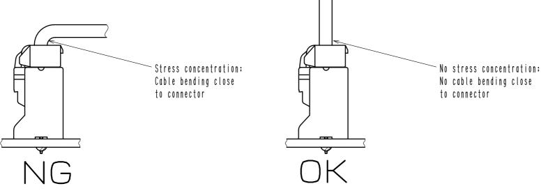
2) When applying load to connector end, please use the retainer for reducing the stress affection on the connector. Retainer shall be installed after inserted crimping contact completely. It might be impossible to insert it when terminal installation is incompleted.
