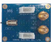
BF4M High Speed Transmission Board : RX2
