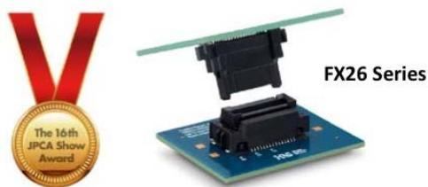
FX26 Series is a floating board to board connector having 140°C heat resistance and high vibration resistance. This series was developed for internal connection of automotive powertrains including inverter and motor control which are key parts of EV and HEV.
