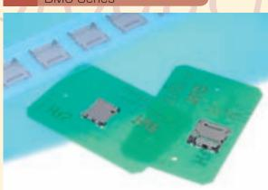
The DM3 series card connectors are adopted by major mobile phone manufacturers as micro SD card connectors. We have newly added the DM3C (hinged type) and DM3D (push-pull type) series to the DM3 family.
