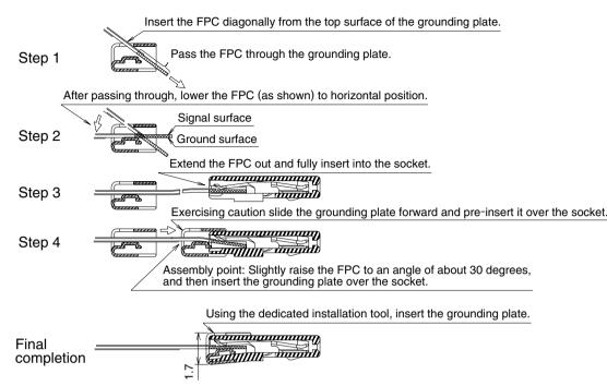
Note 1: The grounding plate and the plug are supplied as separate components.
