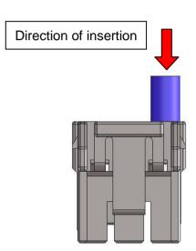
To maintain performance reliability, do not tilt crimped terminals for insertion.
