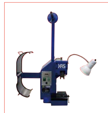
Automatic crimping press (Type CM-105C)
