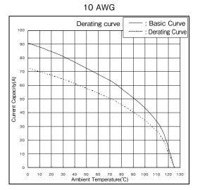
Note 1: The derating curve is a curve is derived by multiplying the basic curve by the derating factor of 0.8.
