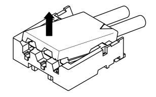
Dlift up to the upper direction and positive lock is released. Removal completes.
