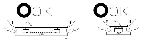
(2) If the connector common be un-mated parallel it can be removed diagonally from the pitch direction. Be careful to do so since this action applies stress on the contact.
