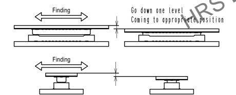
(2) When quiding, the connectors are aligned parallel to each other, with longitudinal and lateral movements restricted. Mate them properly by applying force in this condition.
