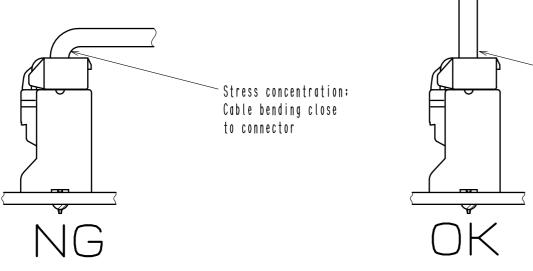
2) When applying load to connector end, please use the retainer for reducing the stress affection on the connector. Retainer shall be installed after inserted crimping contact completely. It might be impossible to insert it when terminal installation is incompleted.
