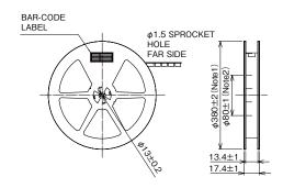
Note1:The (53) specification is  $\phi$ 180 $\pm$ 2. Note2:The (53) specification is  $\phi$ 60 $\pm$ 1.
