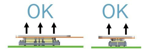
2. If difficult to remove, extract the connector diagonally in the direction of the pitch. Note that removal from the widthwise side will apply a large load to the contacts. When removing from the width direction, pull the end of the FPC in the upward direction. (When a force is applied in the horizontal direction, a large load is applied to the contact.)
