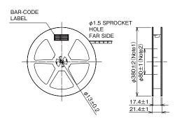
Note1:The (53) specification is  $\phi$ 180±2. Note2:The (53) specification is  $\phi$ 60±1.
