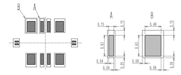
Connector lead on PAD layout
