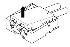
③Lift up to the upper direction and positive lock is released. Removal completes.
