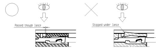
When the cable needs to be pulled for the check, make sure that the applied force is 3 N or lower. Excessive pulling of the cable may damage the housing lance, resulting in the deterioration of the lance retention force.
